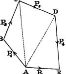
by their resultant AD, that is, the forces AB, BC, CD may be replaced by their resultant AD, and lastly, AD, DE may be replaced by their resultant AE; therefore AE represents the resultant of the given forces in direction and magnitude.
